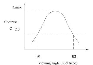
Note: Optimum viewing angle with the naked eye and viewing angle  $\theta$  at Cmax. Above are not always the same
